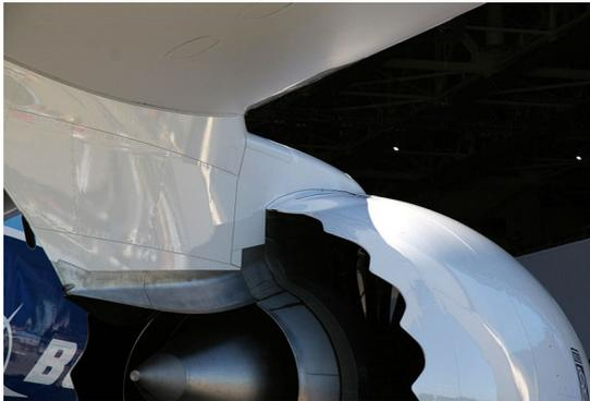
Figure 1.6: Chevron nozzle on a Boeing 787's jet engine.<sup>3</sup>
