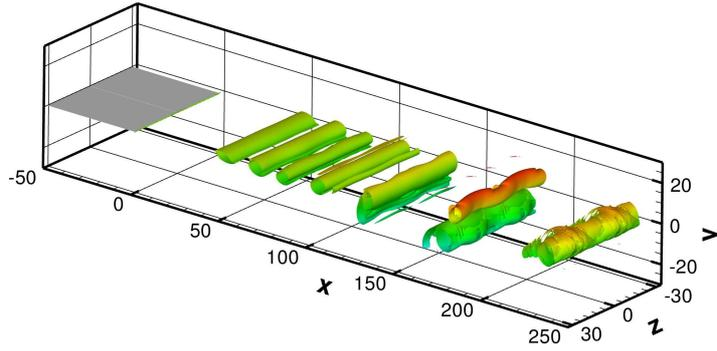
**Fig. 1** Flow structures for the reference case with straight trailing edge, visualized by the isosurface  $\Lambda_2 = -0.001$  along two spanwise periods. Grey scales indicate the wall-normal distance.
