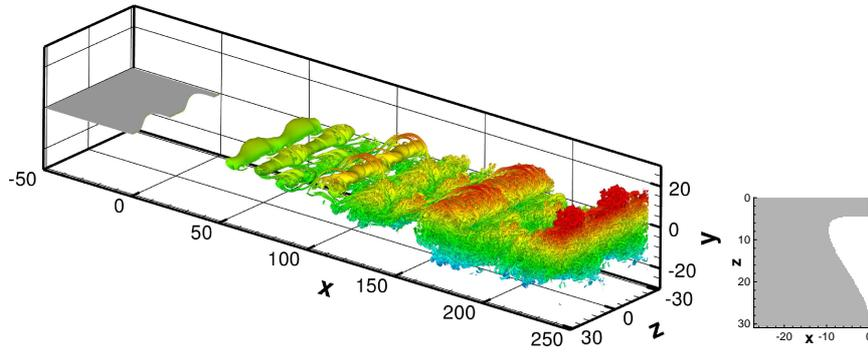
**Fig. 2** Snapshot of the vortical structures due to the non-symmetrical serration ( $\Lambda_2 = -0.005$ ).
