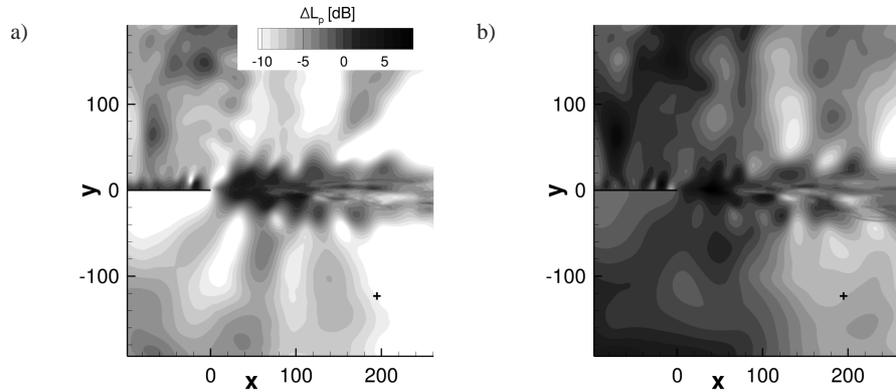
**Fig. 8** Reduction of the overall sound-pressure level in dB compared to the reference case: a) non-symmetric serration and b) narrow rectangular serration, respectively. The location of the pressure spectra in figure 9 is marked by +.
