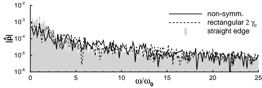
**Fig. 9** Pressure spectra in the farfield ( $x = 195, y = -121.8, z = 0$ ) for the non-symmetric and the rectangular serration with half the spanwise extent, compared with the straight trailing edge in grey.
